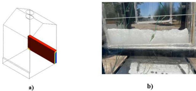
Figure 7. PCM back wall for 3 m/s speed at 2000 s a) numerical modeling b) experimental images
