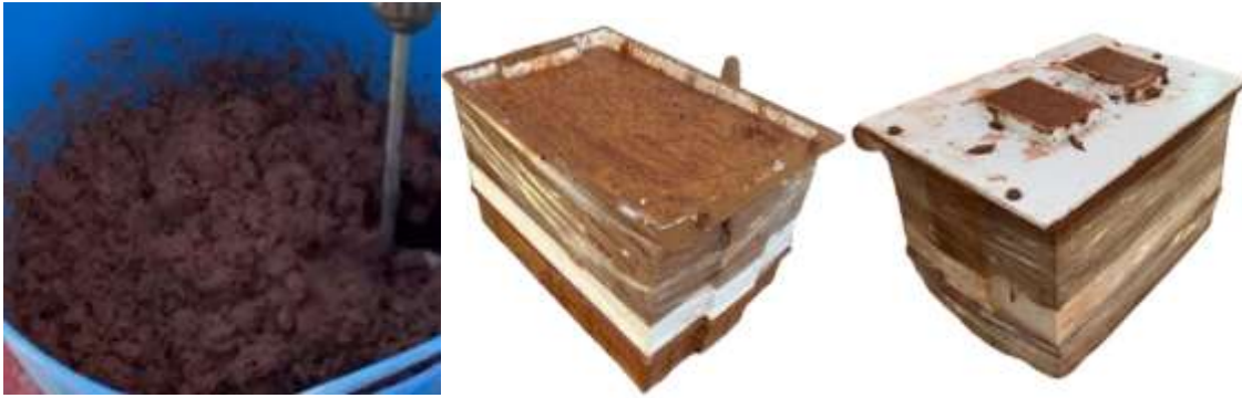
Figure 7. Geopolymer production and placement into a prototype mold
