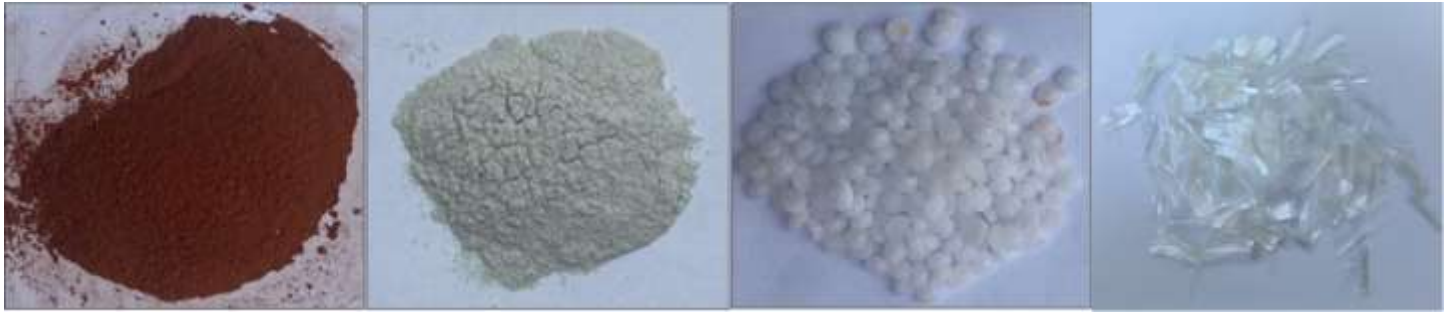
Figure 1. (a) Brick powder, (b) glass powder, and (c) sodium hydroxide (d) micro-synthetic fiber
