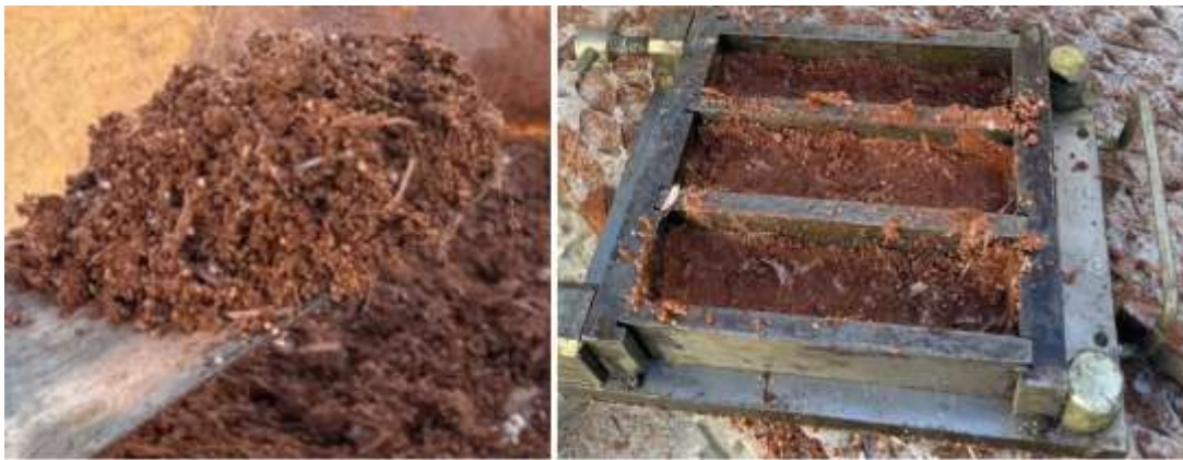
Figure 2. (a) Fresh mixture, (b) prismatic molds (4 × 4 × 16 cm)
