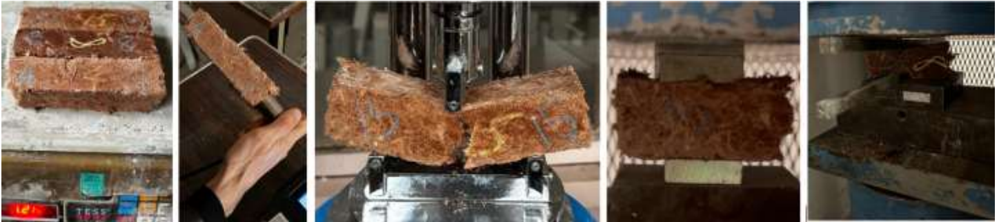
Figure 3. (a) ultrasonic pulse tests, (b) unit weight (c) flexural, (d) compressive, (e) splitting tensile,
